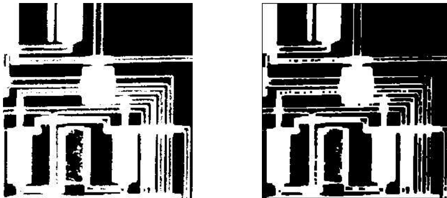
Figure 9.8: Erosion of a binary image
